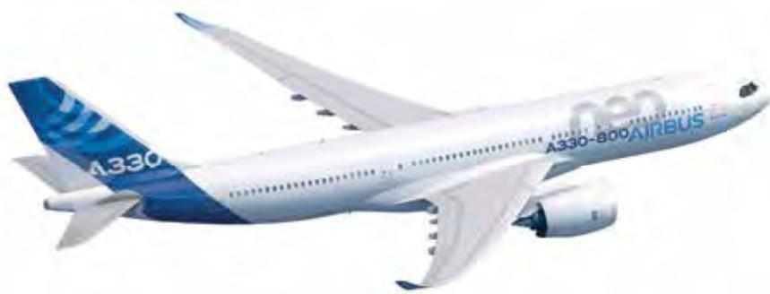
The world's best-selling widebody is now even better. The A330neo has new engines and new wings, bringing a 14% fuel burn efficiency over its predecessor with an additional 400nm range. It also features the new Airspace cabin, which sets a modern benchmark in passenger comfort and wellbeing.
