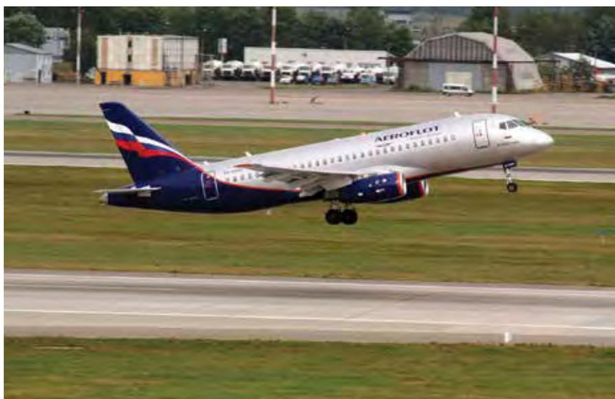
**L**aunched in 2000, the Sukhoi Superjet 100 (SSJ100) is a product of a joint venture between the Russian aircraft manufacturer Sukhoi and the Italian aerospace company Leonardo. It is a new-technology, fly-by-wire regional aircraft powered by two PowerJet SaM146 engines, jointly designed and produced by Snecma Moteurs and NPO Saturn. The aircraft has the highest-ever proportion of western components in a Russian aircraft.
