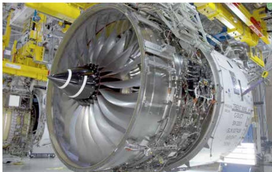
The Trent XWB-97 engine, which powers the Airbus A350-1000
