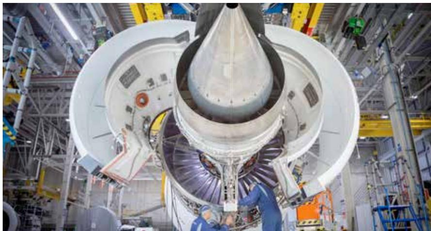
The Trent 7000 engine, which powers the Boeing 787
