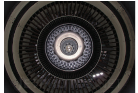
An inside view of the CFM56-5B - a popular engine according to engine investors.
