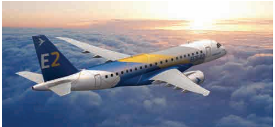
The E195-E2 has been stretched by three seat rows
